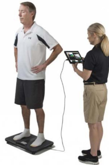
Figure 2. Depiction of the BBT setup. Participants stood with eyes closed, hands on hips and two feet on the BTrackS™ Balance Plate, while BTrackS™ Assess Balance software guided the test administrator through measurement of COP path length over four trials.
